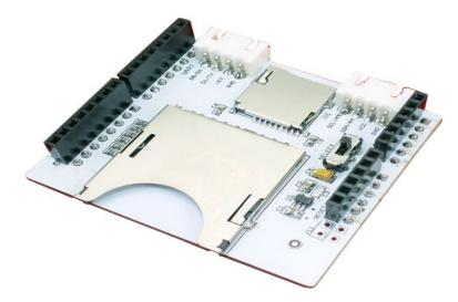
The SD card shield adds storage to your Arduino project. It supports SD, SDHC, or MicroSD TF cards. Use the on-board toggle switch to select the SD card type. And when you want plug a sd card on it, you should select the switch to the right direction.
